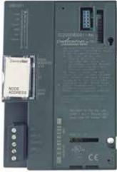
A Remote I/O Unit connects VersaMax I/O modules to a host PLC or computer via a variety of networks. This makes it easy to include VersaMax I/O in the innovative PROFINET interface, as well as Genius, PROFIBUS-DP, DeviceNet, or other Ethernet installations. Together, the Remote I/O Unit and its modules form an I/O station capable of providing up to 256 points of I/O.
